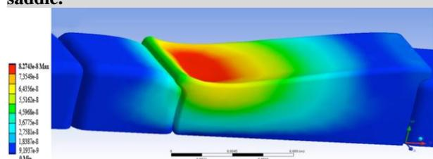
**Figure 9.** Stress distribution in model 2 when the load was applied in the end of the tooth-bounded saddle.
