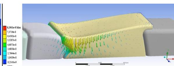
**Figure 8.** Schematic diagram of stress distribution in model 1 when the load was applied in the end of the tooth-bounded saddle.
