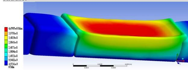
Figure 3. Stress distribution in model 2 when the load was applied in the middle of the tooth-bounded saddle.
