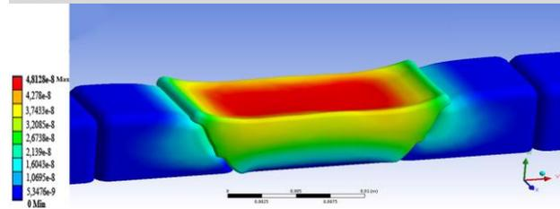
Figure 5. Stress distribution in model 3 when the load was applied in the middle of the tooth-bounded saddle.
