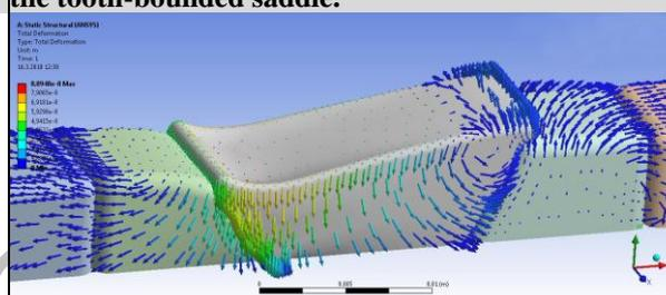
**Figure 12.** Schematic diagram of stress distribution in model 2 when the load was applied in the end of the tooth-bounded saddle.
