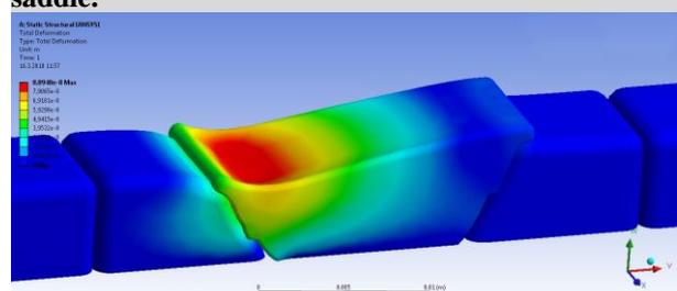
**Figure 11.** Stress distribution in model 3 when the load was applied in the end of the tooth-bounded saddle.
