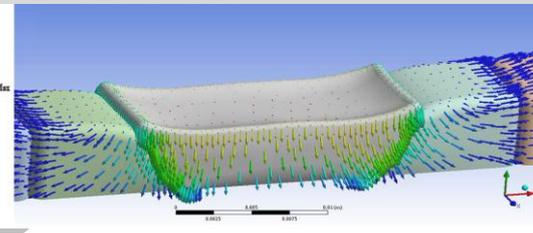
Figure 6. Schematic diagram of stress distribution in model 3 when the load was applied in the middle of the tooth-bounded saddle.
