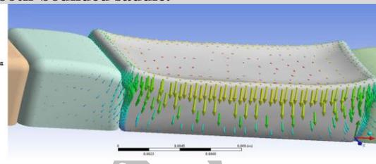
Figure 4. Schematic diagram of stress distribution in model 2 when the load was applied in the middle of the tooth-bounded saddle.
