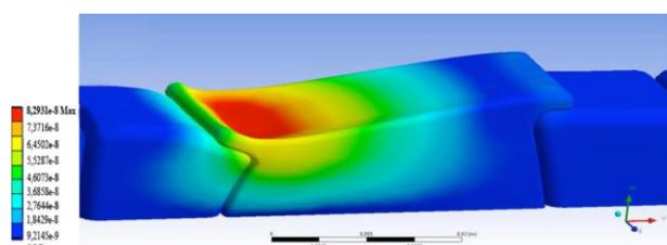
**Figure 7.** Stress distribution in model 1 when the load was applied in the end of the tooth-bounded saddle.
