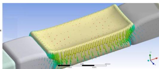
Figure 2. Schematic diagram of stress distribution in model 1 when the load was applied in the middle of the tooth-bounded saddle.
