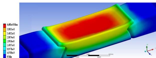
Figure 1. Stress distribution in model 1 when the load was applied in the middle of the tooth-bounded saddle.
