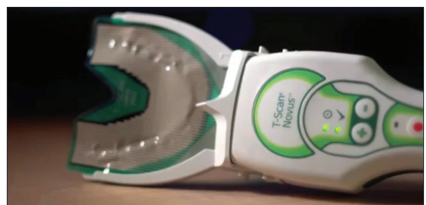
Figure 3. T-Scan III Novus (Tekscan Inc.) handle and sensor film for load registration
