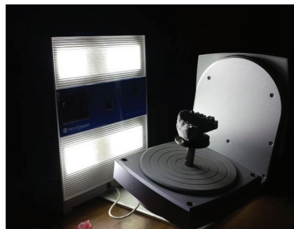
Figure 1. Scanning of a study model positioned on a stand with NextEngine 3D scanner HD (Next Engine Inc., Santa Monica, CA, USA)
