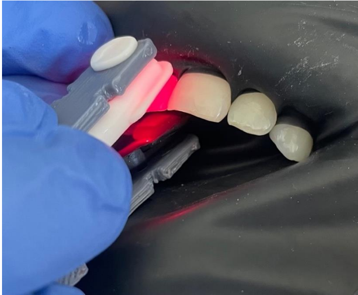
Figure 2. Custom made pulse oximeter dental probe
