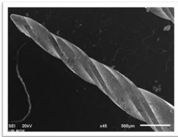
**Figure 4.** SE image K3 instrument (25–0.08), second experimental group (corrosion on the apical third) ( $\times 45$ )
