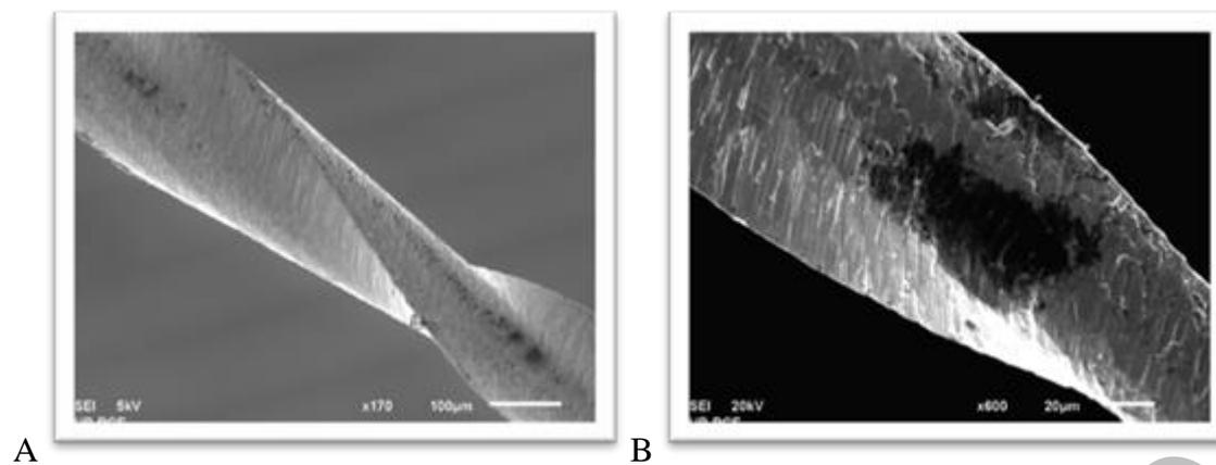
**Figure 1.** Spin echo image of the new Mtwo instrument (10 / 0.4): A – surface of the middle third on which the presence of corrosion is observed ( $\times 170$ ); B – detail from the previous image at higher magnification ( $\times 600$ )
