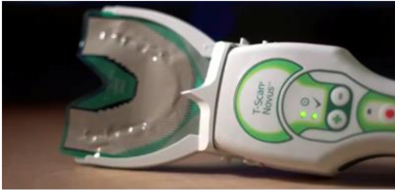
Figure 3. T-Scan III Novus handle and sensor film for load registration
