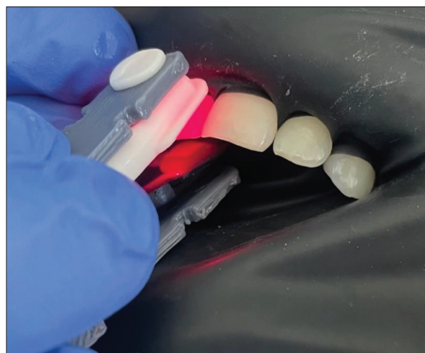
Figure 2. Custom-made pulse oximeter dental probe
