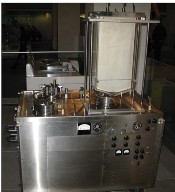
Figure 2. Heart–lung machine dating from 1958 (design first appeared in 1955), used in London's Middlesex Hospital
