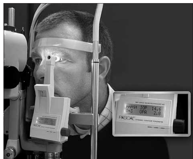
Figure 3. DCT measuring of IOP with presented display data
